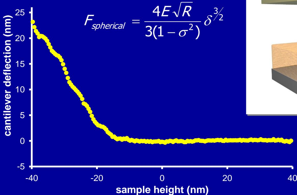
We measure  $\delta$ . Knowing  $R$  (tip radius) and  $\sigma$  (poisson ratio  $\sim 0.5$ ) we can solve for the Young's Modulus ( $E$ ), which is related to 'crosslink' density
