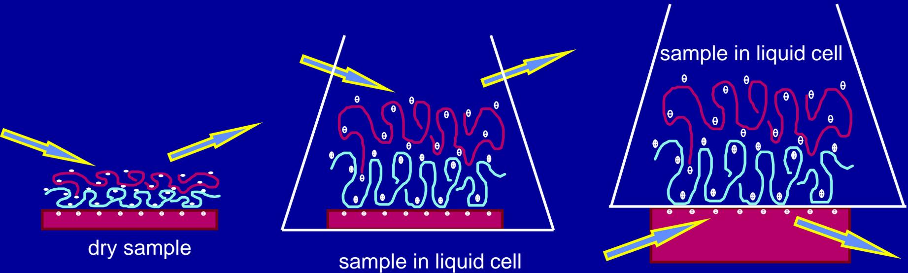
"Variable temperature, 0-100% humidity, and liquid neutron reflectometry sample cell for biomimetic materials."
