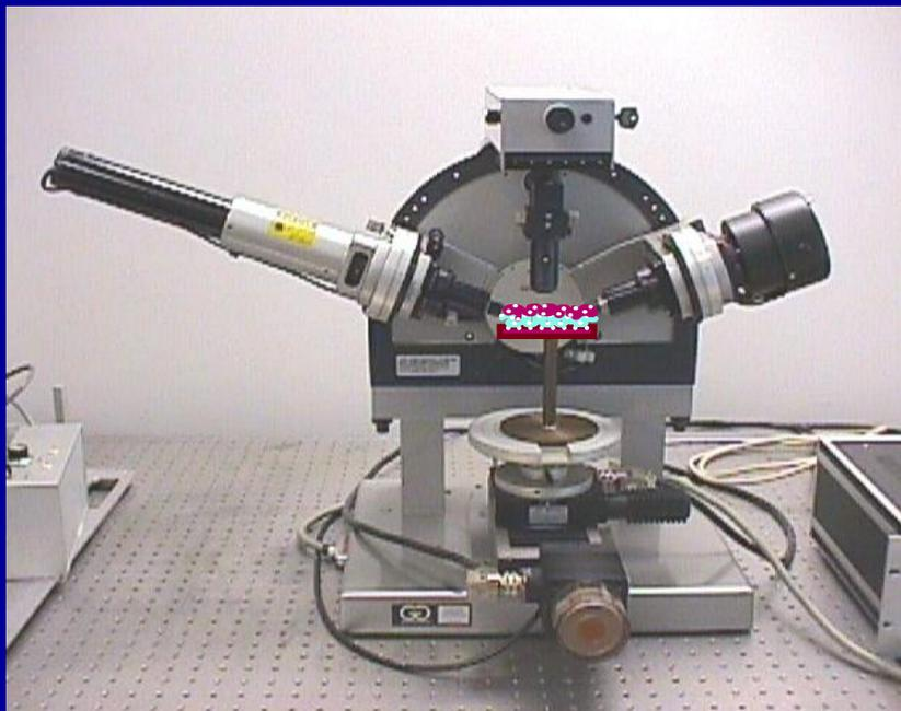
Using *in situ* ellipsometry to measure layer thickness :
