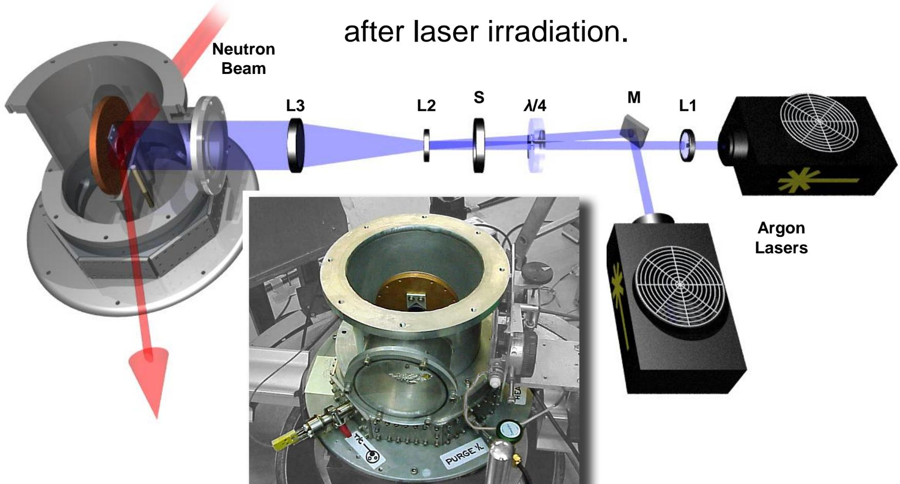
Ellipsometry can only measure *average* density however, but, we can use variable angle neutron reflectivity :
