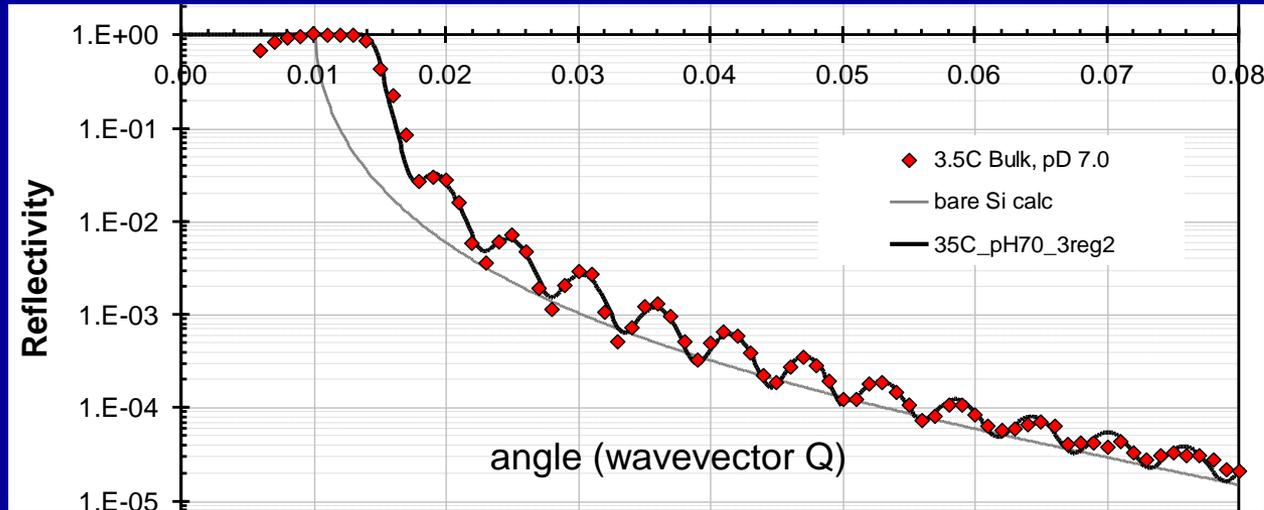
Now use neutrons wavelength  $2.4\text{\AA}$ . Measure reflected intensity as incident angle is increased.
